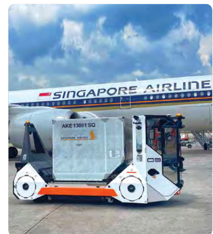
Changi Airport is the first in the world to test the Auto-DollyTug's ability to autonomously load and unload ULDs at the aircraft stand.
